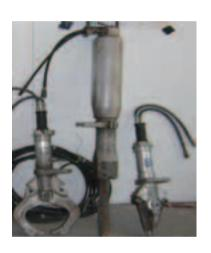
Portable splitting and bursting machines, which are used in concrete demolition works that are performed bursting
