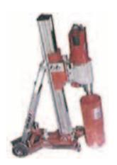
Coring machines, which are used in concrete demolition works that are performed by core drilling
